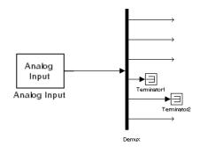
Depending on the board and the number of channels used, I/O conversion time can affect the maximum sample rate that can be achieved on your system. Rather than converting unused channels, we recommend specifying only the set of channels that are actually needed for your model.
