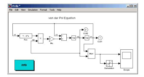
The Simulink model rtvdp.mdl window opens.
